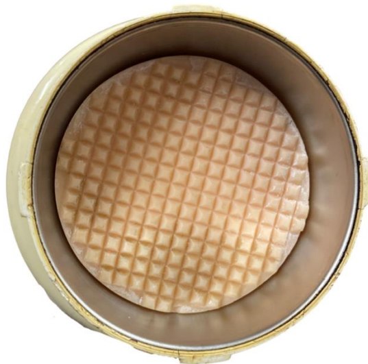
Figure 18: Cross-hatch spheronizer plate
